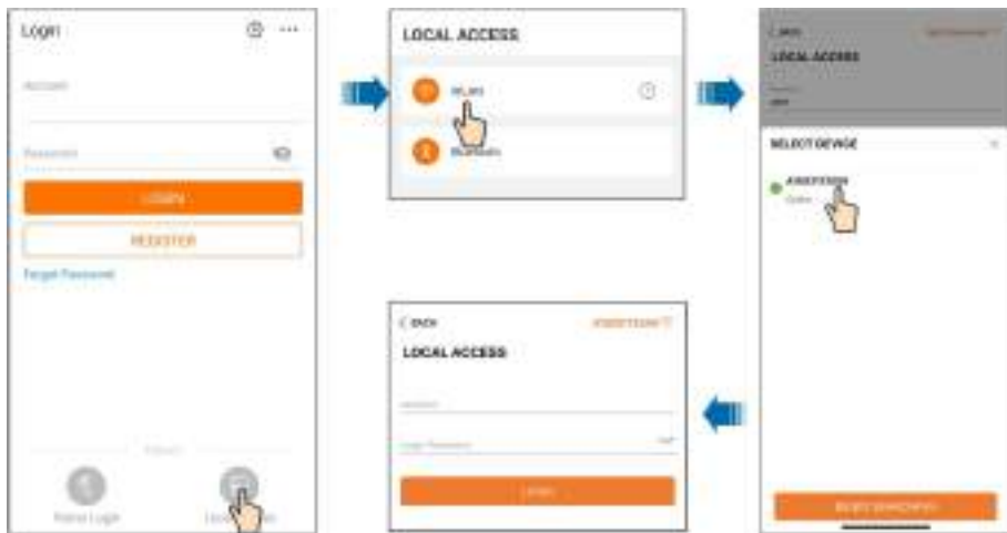
Figure 7-3 WLAN Local Access
