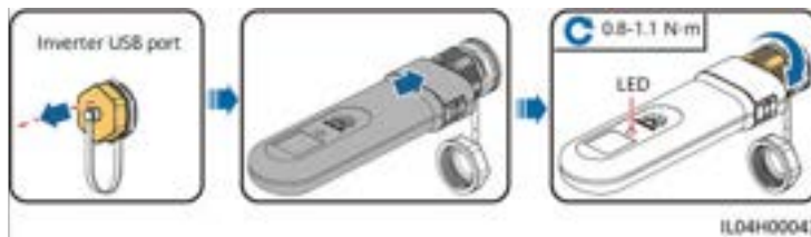
Figure 7-9 Installing the Smart Dongle
