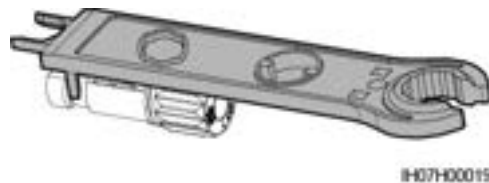
Figure 5-14 Removing a DC connector
