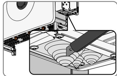
8. Guide the cable through the sealing plate into the device and fasten the protective cover screws (TX30, tightening torque: 4.2 Nm to 4.5 Nm) to the bottom of the inverter.
