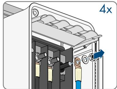
6. Loosen the grounding conductor and the ring terminal lug using a ratchet.
