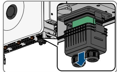
3. Remove the swivel nut from one of the cable glands for the communication cable.
