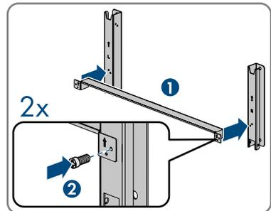
2. Align the mounting bracket using a spirit level and mark the drilling positions.
