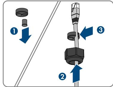
7. Press the two-hole cable support sleeve with the cable into the cable gland and route the network cable to the RJ45 connection at the bottom of the cable compartment. Ensure that any unused enclosure openings of the two-hole cable support sleeve are sealed with sealing plugs.
