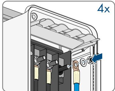
12. Place the grounding conductor incl. 1 washer and hex nut onto the stud bolt in the middle section. Now tighten it all using a ratchet.
