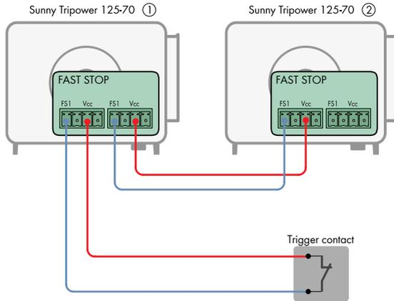
Figure 10: Circuitry overview for connecting a contact for the fast stop and the connection of several inverters
