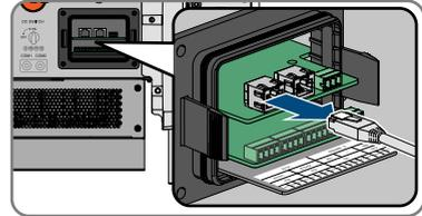
13. Remove the connection cable from the cable gland.
