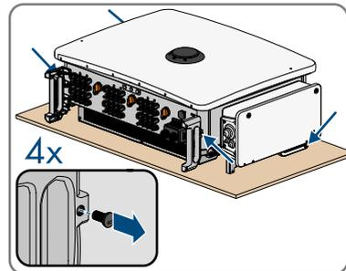
6. If the inverter is to be hooked into the mounting bracket using a lifting gear, screw the eye bolts into the 2 upper threaded holes on the right-hand and left-hand side of the inverter and attach the lifting gear to them. The lifting gear must be suitable to take the weight of the inverter.
