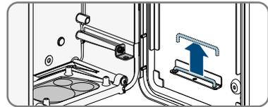
4. Engage the end of the limiting lever in the cable compartment with the thread.
