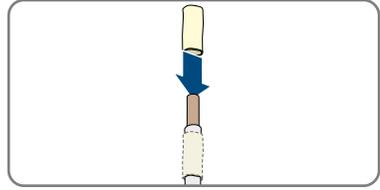
2. Plug the terminal lug onto the conductor.
