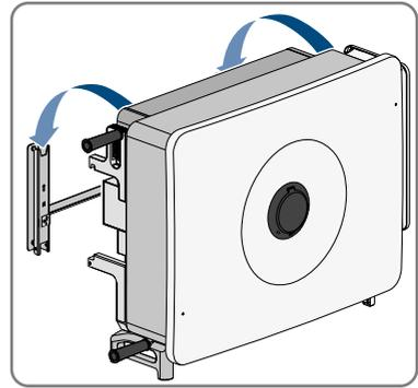
9. Remove all 4 carrying handles from the threaded holes or remove the eye bolts of the lifting gear and once again screw in the sealing screws (flat-blade screwdriver 4 mm, tightening torque: 2 Nm).
