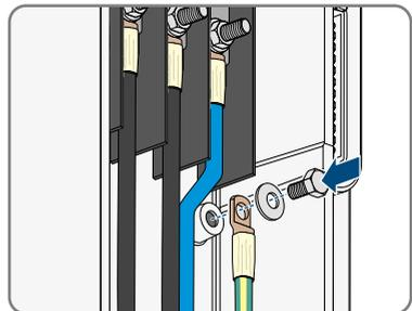
13. Ensure that the AC cable is not under tension.
