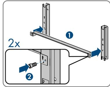
2. Align the mounting bracket using a spirit level and mark the drilling positions on the profile rails.
