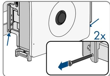
6. Unhook the inverter from the mounting bracket.
