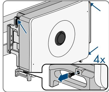
2. Screw all 4 carrying handles or the eye bolts of the lifting gear into the threaded holes.
