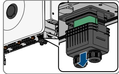
12. Remove all connection cables from the communication assembly.
