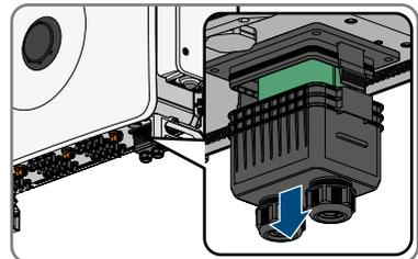
6. Remove the swivel nut from an unused cable gland for communication cables.
