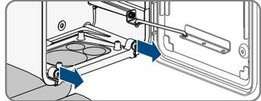
3. Pull the AC seal plate with cassette out of the guide.
