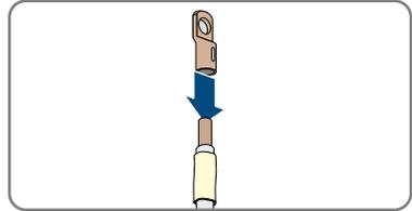
3. Insert the stripped section of the insulated conductor into the ring terminal lug and crimp using a crimping tool.
