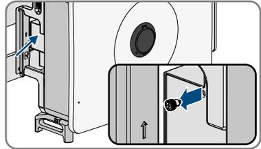
4. Remove the sealing plate of the fan cassette.
