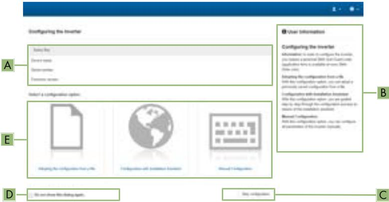
Figure 11: Layout of the **Configuring the Inverter** page
