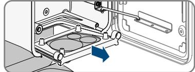
4. Loosen the 4 screws of the AC sealing plate attached to the inverter at delivery (TX30) and remove the AC sealing plate.
