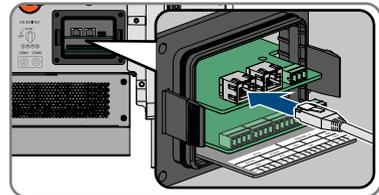
9. Ensure that the RJ45 connector is firmly seated and that there is no tension on the cable.
