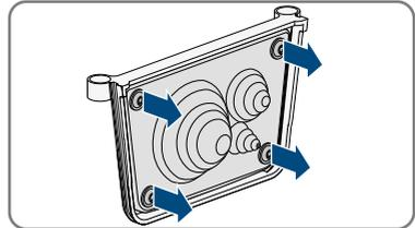
5. Ensure that the AC device opening is free of contamination.
