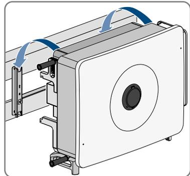
9. Remove all 4 carrying handles from the threaded holes or remove the eye bolts of the lifting gear and again screw in the sealing screws using a flat-blade screwdriver (4 mm, tightening torque: 2 Nm).
