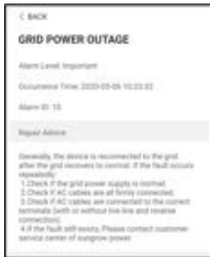
figure 7-9 Detailed Fault Alarm Information
