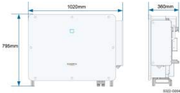
figure 2-3 Dimensions of the Inverter(in mm)
