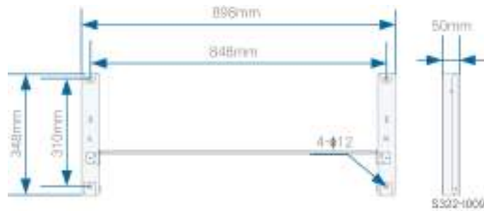
figure 4-1 Dimensions of mounting-bracket
